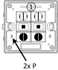
②nd wall switch: press P button one time
