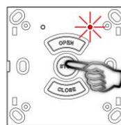
select (to be removed) channel A or B and press CLOSE button:
