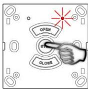
hold the remote within 2 meter from receiver. Select channel A or B and press OPEN button:
