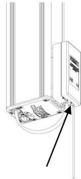
press and hold the program button for 10 seconds until control led starts blinking
