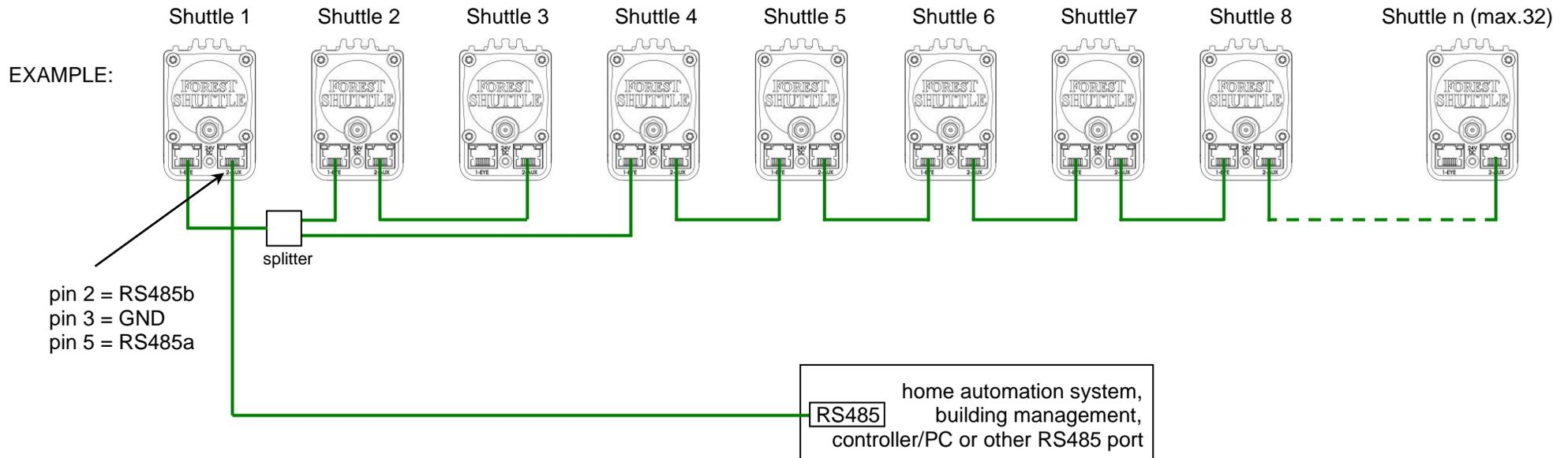
All Shuttles have standard the address 'OWN'. This address can be changed to a unique address before connecting to the FX-bus. Commands are addressed directly to a Shuttle or, in some cases, globally to the entire bus. In order to get a response message from a Shuttle (position ect.) you need to send a request to a unique address. The addressed motor will then respond with a message onto the bus to the Home Automation system / Controller / PC.
