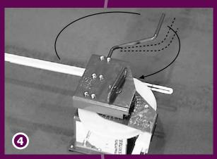
Insert the Guide-Wedge (B) firmly into the place between the metal part of the Bending Dye (C) and the track to position the track in the right place. Take the measurement of the first curve from the end of the Metal House (E) to the end of the track. This will create the distance from the outside of the track to the wall. Start curving by turning the handle (H) clockwise.
