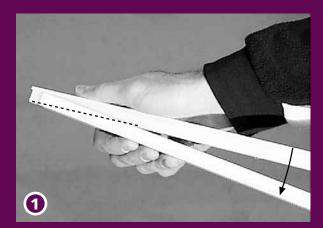
Press Bending Strip (A) into slot of the track, where you want to make a curve. Do not slide the strip in: this reduces the lifetime of the nylon strip.
