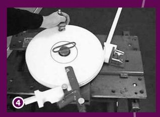
Tighten the screw on the Guide-Wedge. Start bending by turning the handle until the required angle is reached. For two curves in one track, measure from the outside of the track to the measurement line (F). This will create the distance from the outside of the track between the two curves.
