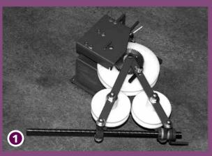
Remove the Metal Pin (C) and the regular bending dye from the Compact Bending tool. Insert the Continuous Curver with the unit Stabilizer (D), so that slack between the Small Bending Dyes (A) and the Compact Bending tool will be avoided.
