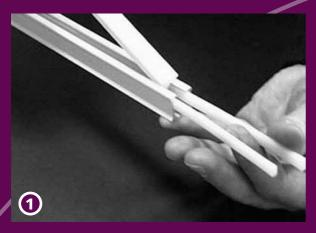
First, insert the two smaller bending strips into the track. Then, press the bigger bending strip into the slot of the track between the smaller ones.
