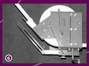
When angle is unknown, use the Metal Protractor (G) and place it against wall or on mal.
