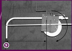
To make a second curve of 90° in the same KS-track, use a tape measure from the outside of the track to the measurement line. This will create the distance from outside to outside of the two curves.
