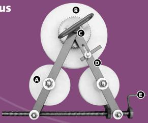
The Continuous Curver can be used when curves with a radius other than 10 cm (4") have to be made, like bay windows, arches, bows and circles. When using this option frequently, consider the purchase of the Electric Bending Machine.
