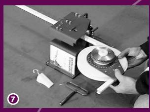
When the required curve is made, turn the handle (H) a few times anti-clockwise to release tension. Then, remove the Guide-Wedge, Metal Pin (D) and slide-out the Bending Dye from the Metal Housing, together with the track.
