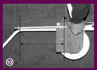
For curves, other than 90°, use a reference point in the middle of the first curve. For the second curve, use the Measurement Line. This will create the distance from center to center of the two curves.
