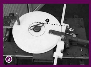
Place the Guide-Wedge (C) as depicted on the foto. Slide the track in position and determine the required size from the measurement line (F) to the end of the track. This will create the distance from the outside of the track to the wall.
