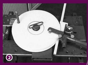
Insert the track from the backside of the Bending tool, between the Bending Dye (A) and the Bending House (E). Place the handle (D).
