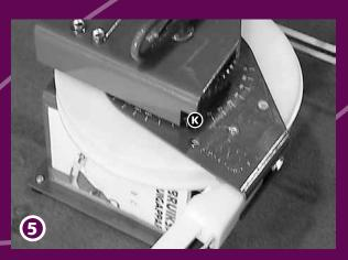
Continue until the required angle has been reached. The Arrow (K) points exactly to the required angle on the scale divider. Turn a few degrees more to avoid spring back of the aluminium track.
