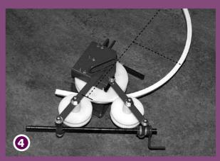
Run the whole distance to be bent through the Continuous Curver until the reference points hit the first Small Bending Dye (A), each time. The radius needs to be checked frequently. If the radius is still not achieved, turn the Small Handle a few times more. Repeat this, until the required radius is created. It is possible to reverse the curve, once the radius is overbent.
