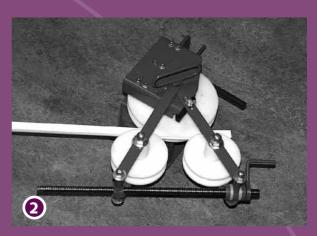
For determining necessary track length 3,14 x diameter of the circle. Add 10 cm (4") more on both ends. Insert the bending strip into the track. Place the track between the Bending Dyes (A and B) with its slot facing up to make a right hand curve, or down to make a left hand curve. Turn the small handle (E) a few times to avoid slack.
