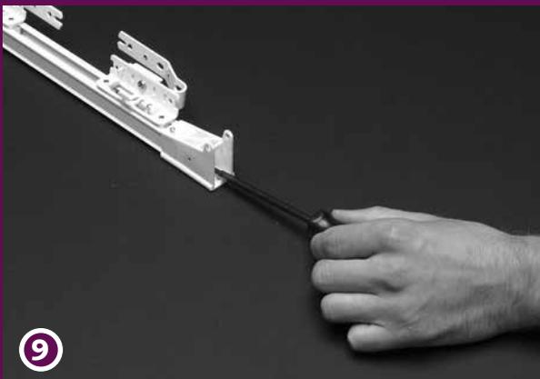
9 Ensure that the cord runs behind the metal pin in the pulley. This avoids slack in the mechanism during operation.
