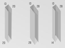
small channel regular channel ventilation channel Please note: With larger surfaces from approx. 2m<sup>2</sup>, the film may be pushed out of the channels by the heat trapped between the glass and the film (generally in case of narrow and tall systems), which is when it is advisable to use ventilation channels (see illustration)
