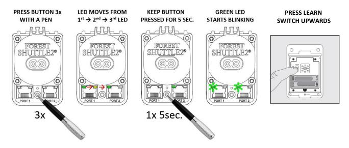
You can test the connection by pressing the grey start-button on the back of the sensor shortly. This will send the RF OPEN command. Deleting a sensor from a programmed Shuttle: same action as programming, only press LEARN button downwards.
