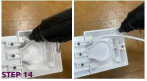
Put a small drop of instant glue on the back of the connector.
