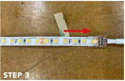
Carefully slide the LED strip into the strip into the connector as shown above.
