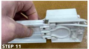
Carefully slide the motor pulley into the track, whilst keeping the connector in place with your finger.
