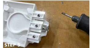
With a rotary tool (e.g.) Dremel carve a bit of the motor pulley
