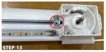
Slide the metal clip in place and tighten the screw.
