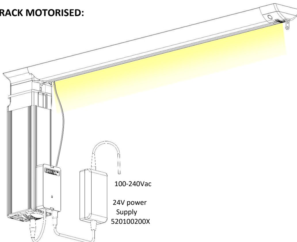
Choose the power supply according to the length of the DS-XL LED track (no difference for Shuttle S/ECO and Shuttle M):
