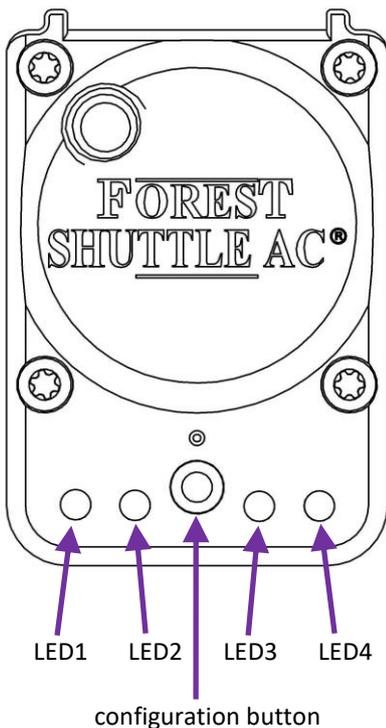
Use a pin to change settings in the configuration menu. Choose the setting you want to change (table below) and press the button that many times (corresponding with setting).
