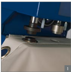
1. Combined cutting and pressing
